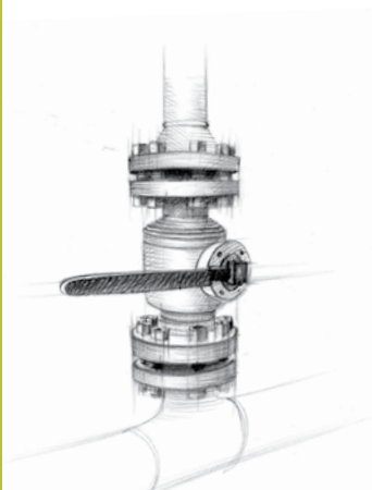
Ball valve of gas separator piping of first gas collection point
